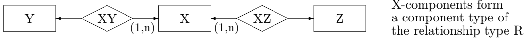
FIGURE 4.4: The ER Representations of a Multivalued Dependency for a First-Order Relationship Type
